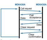
Frame relay measurement sequence
